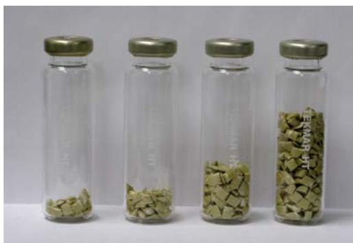
Figure 1 – Comparison of 1 g, 2g, 4g, and 8g of a HT Polymer Sample in 22 mL High Temperature Headspace Vials
