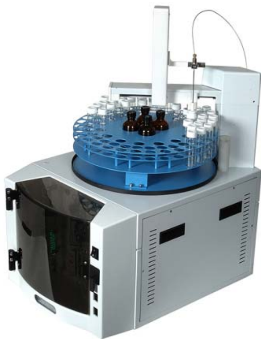
Figure 1. The Fusion uses four Boston round bottles (125mL) in its autosampler's center position for calibration, calibration verification and system suitability analysis.
