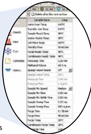
Other parameters that are common to all methods are seen here and are user selectable with recommended default values and an intuitive prompt that indicates min and max allowable values as well as the variable description.
